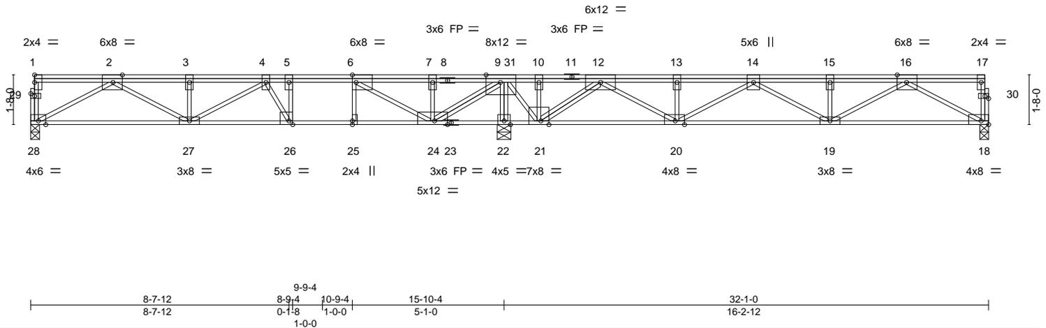
Plate Offsets (X,Y)-- [2:0-3-12,Edge], [6:0-1-8,Edge], [9:0-5-12,Edge], [16:0-3-12,Edge], [18:Edge,0-1-8], [20:0-3-12,Edge], [21:0-3-4,Edge], [24:0-5-4,Edge], [25:0-1-8,0-0-0], [26:0-1-8,Edge], [29:0-1-8,0-1-0], [30:0-1-8,0-1-0]
