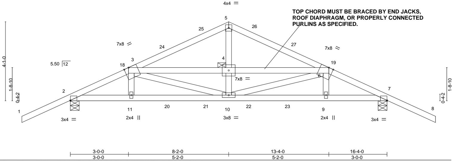
**TOP CHORD MUST BE BRACED BY END JACKS, ROOF DIAPHRAGM, OR PROPERLY CONNECTED PURLINS AS SPECIFIED.**
