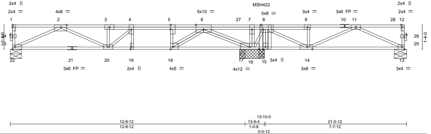
Plate Offsets (X,Y)-- [2:0-3-12,Edge], [5:0-3-0,0-0-0], [6:0-5-0,Edge], [8:0-1-8,Edge], [12:0-1-8,Edge], [14:0-3-4,Edge], [18:0-1-8,Edge], [19:0-1-8,Edge], [23:0-1-8,0-1-0], [25:0-1-8,0-1-0]
