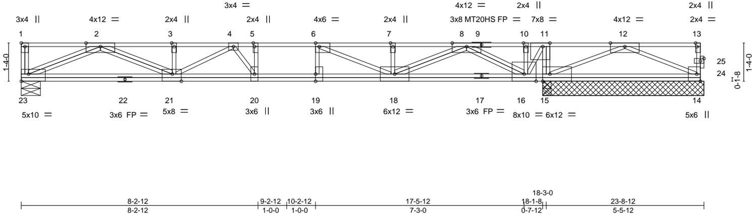
Plate Offsets (X,Y)-- [1:Edge,0-1-8], [5:0-1-8,Edge], [6:0-1-8,Edge], [11:0-3-0,Edge], [13:0-1-8,Edge], [15:0-3-0,Edge], [19:0-3-0,0-0-0], [21:0-3-12,Edge], [23:Edge,0-3-0], [24:0-1-8,0-1-0]
