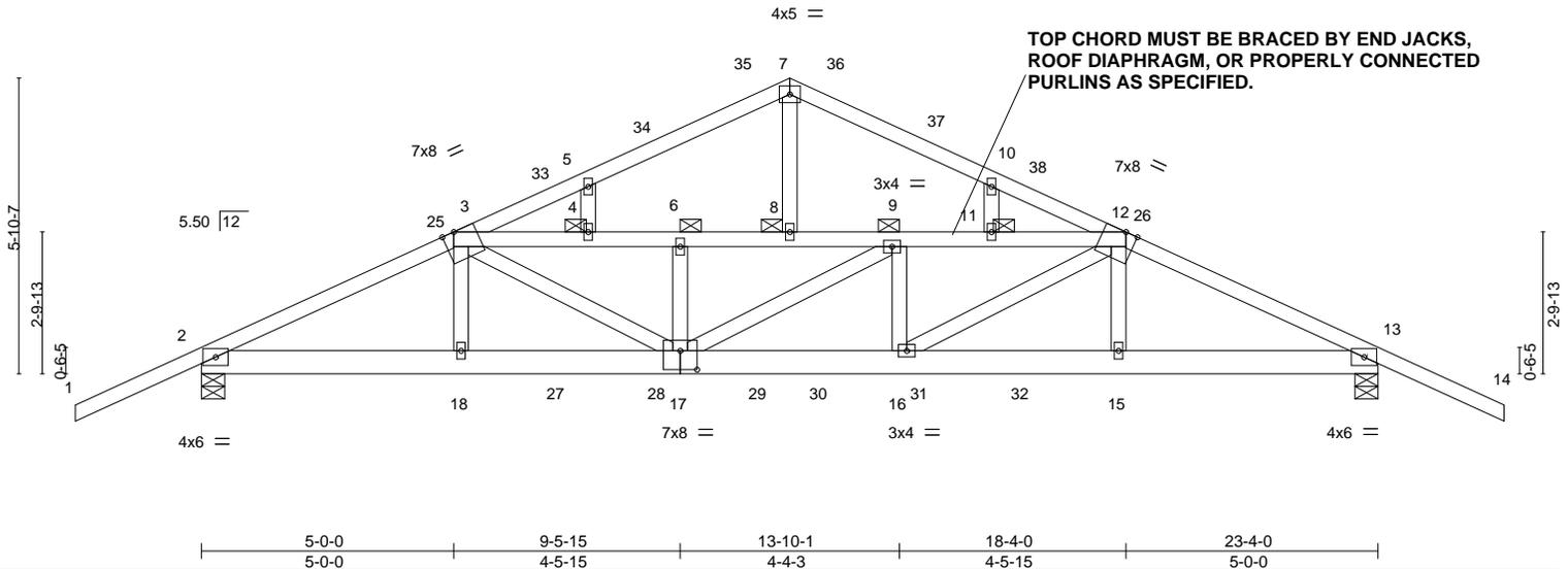
**TOP CHORD MUST BE BRACED BY END JACKS, ROOF DIAPHRAGM, OR PROPERLY CONNECTED PURLINS AS SPECIFIED.**
