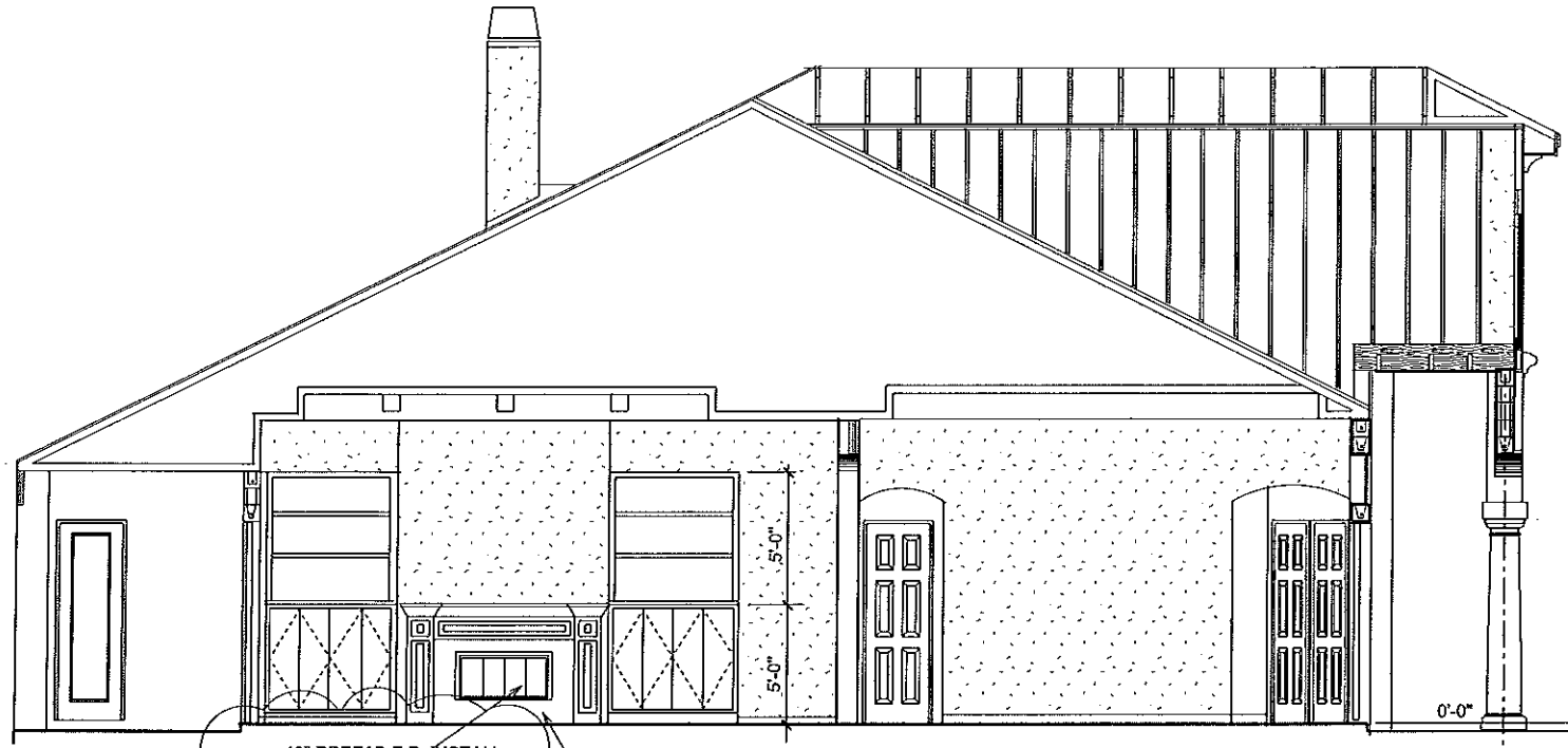
42" PREFAB F.P. INSTALL PER MANUF SPECS INCLUDING OUTSIDE AIR SUPPLY 12" GRANITE SURROUND FIREPLACE ELEVATION
